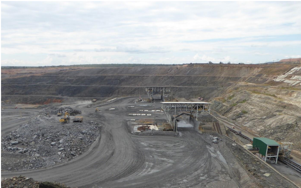
Figure 16-5 Trolley assisted waste haulage in Sentinel Pit, Q4 2019
