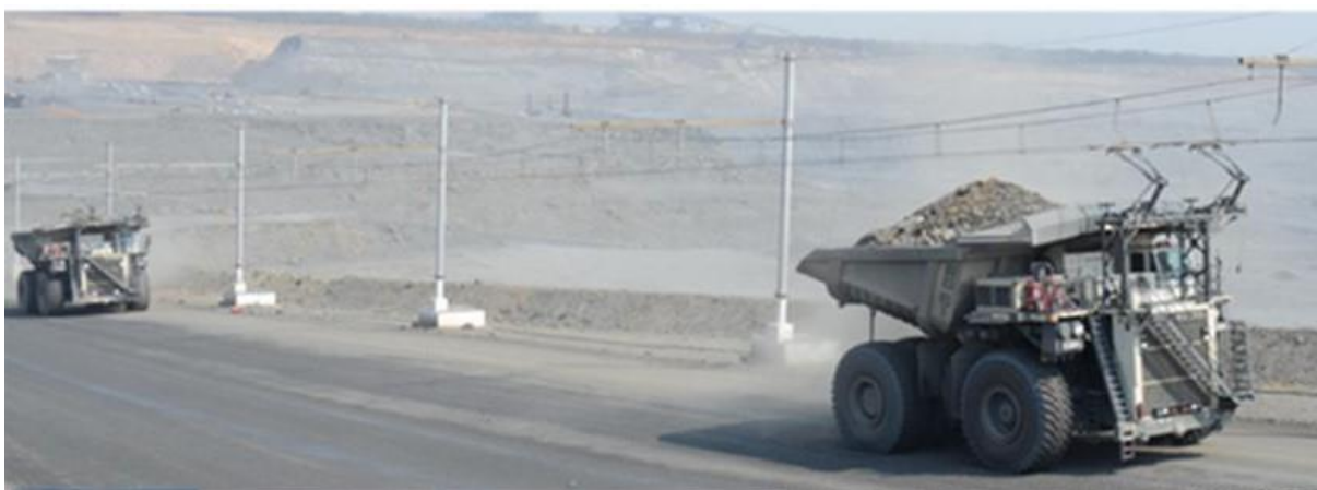
Figure 16-5 Trolley assisted waste haulage in Sentinel Pit, Q4 2019
