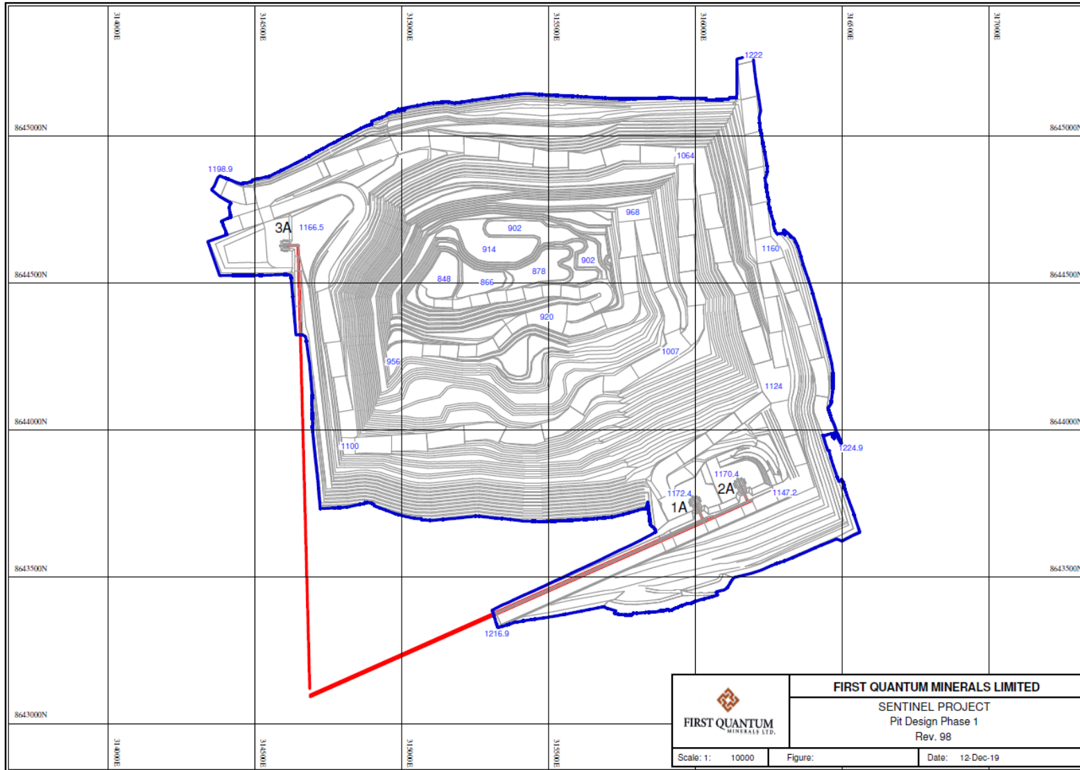
Figure 15-11 Sentinel Phase 1 pit design and IPC positions
