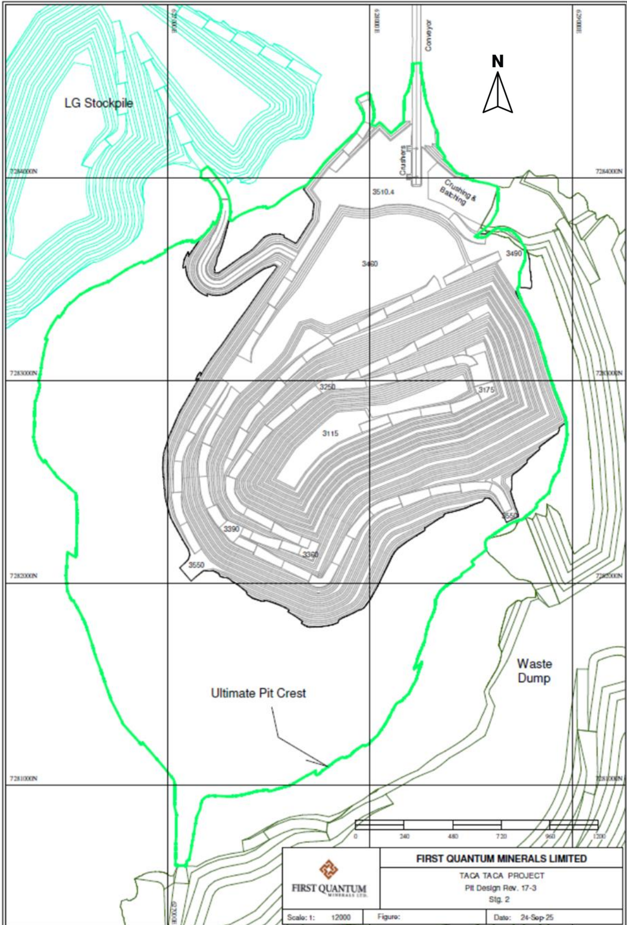
Figure 15-14 Taca Taca Stage 2 design pit
