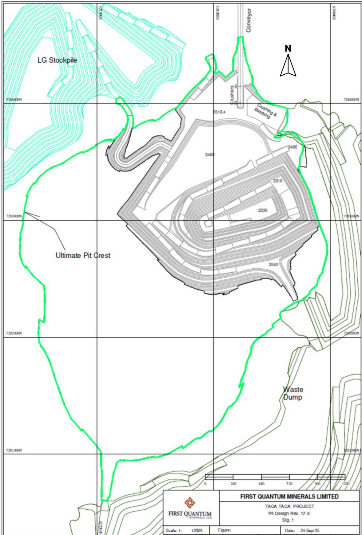
Figure 15-13 Taca Taca Stage 1 design pit
