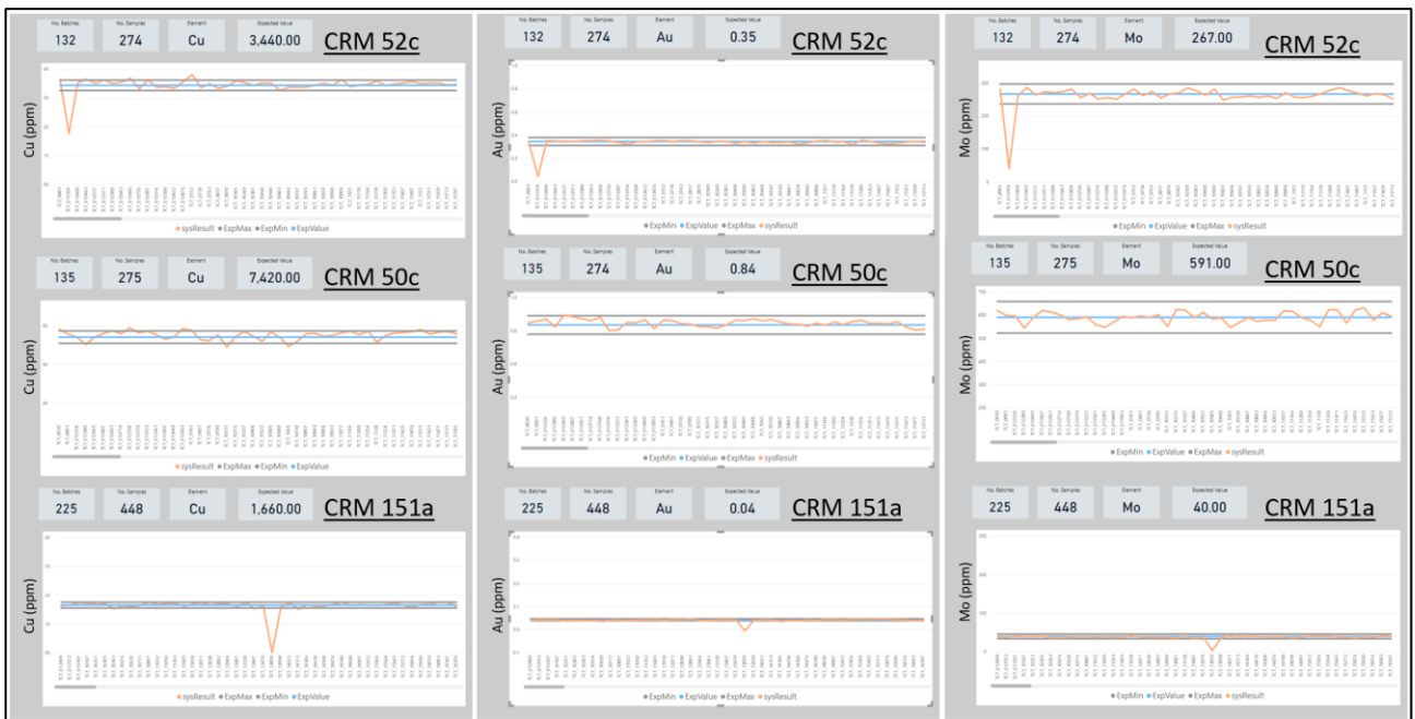
Figure 11-9 Control charts showing Cu, Au, and Mo results from the 3 CRM samples analysed during Lumina diamond drill campaign
