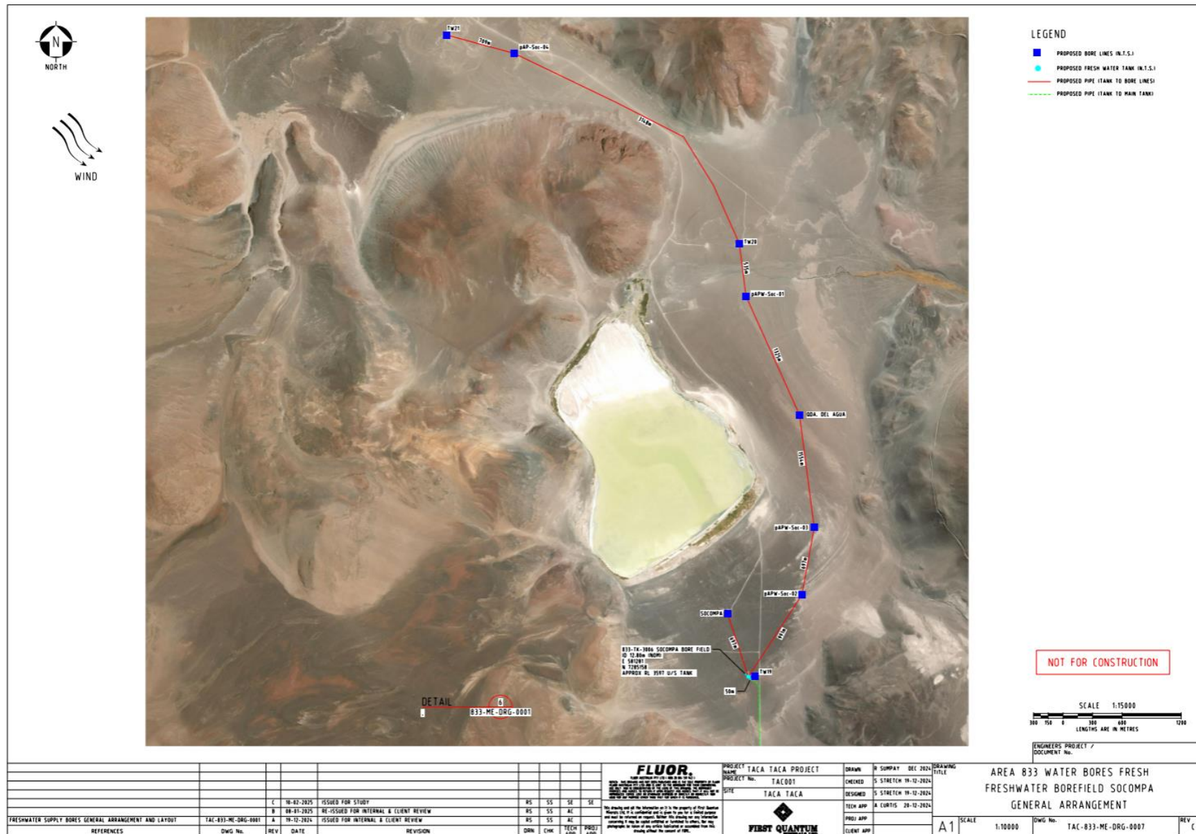
Figure 18-8 Layout of Socompa borefield (source: Fluor, 2024)
